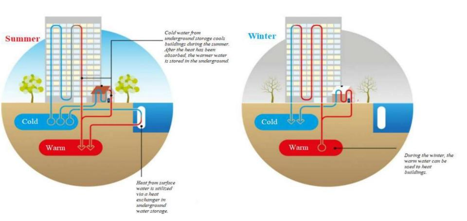
TEO is usually combined with Aquifer Thermal Energy Storage (ATES) in the subsoil
