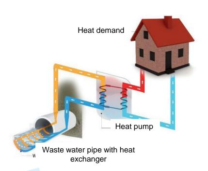
In sewer pipes, pressure pipes, effluent pipes
